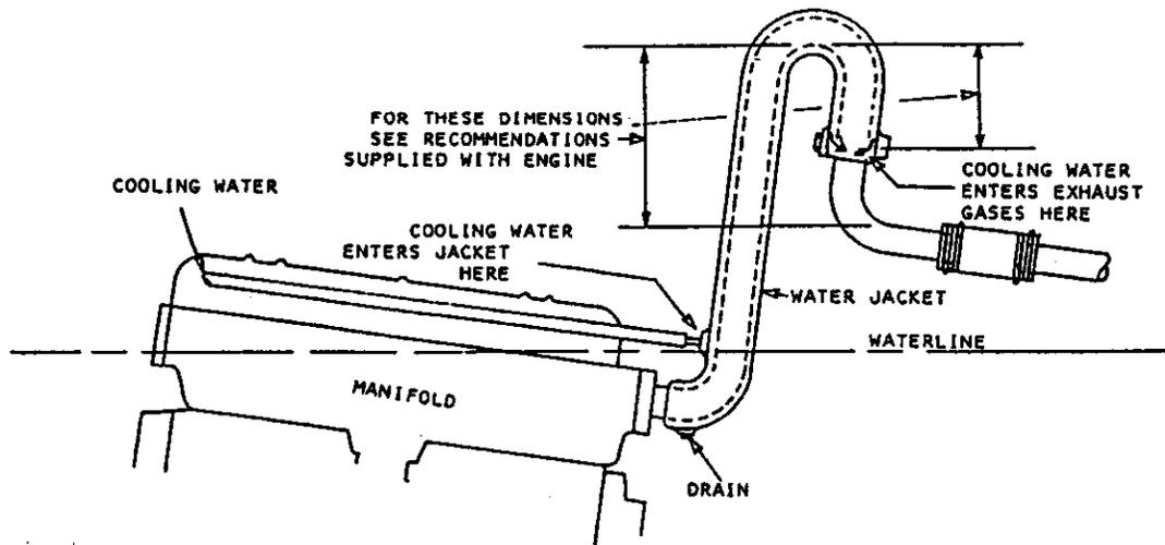
**FIGURE 3 - TYPICAL EXHAUST RISER**
