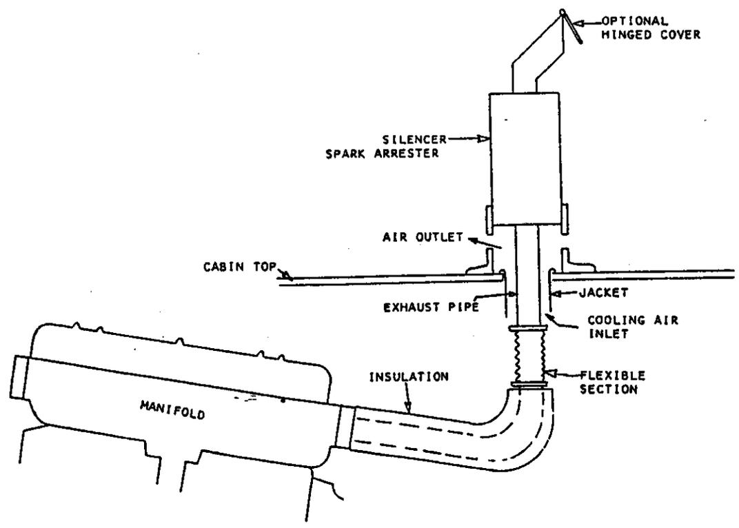
**FIGURE 5 - TYPICAL WATERLIFT EXHAUST SYSTEM**
